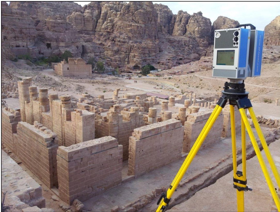
Scanning the Great Temple with a Z+F scanner
