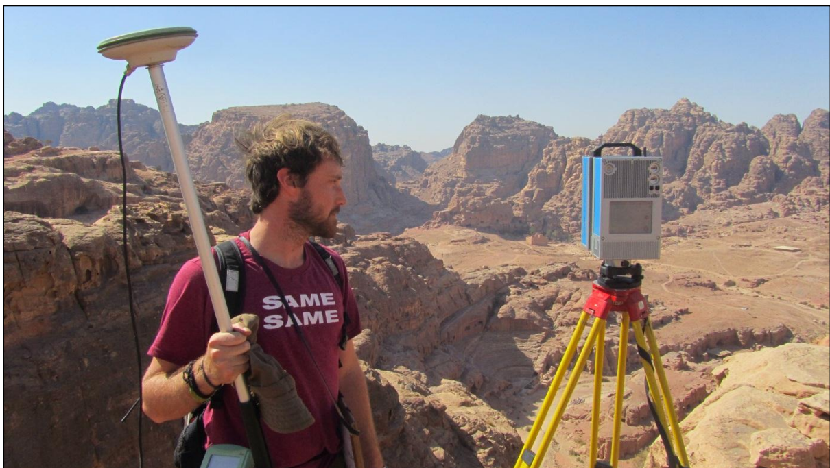
GPS survey and scanning on top of the Siq
